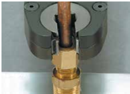
Make sure that the socket is set to the open position. If not, push the throttle lever down half way to release the socket back to the open position.
