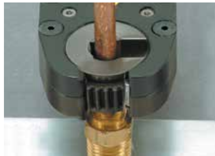
Slide the tool on the fastener and push the throttle lever down fully to run the fastener down.
